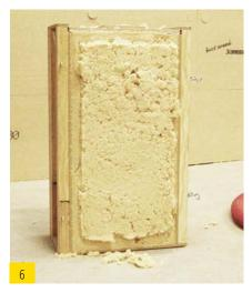
Open test element and assess filling result
