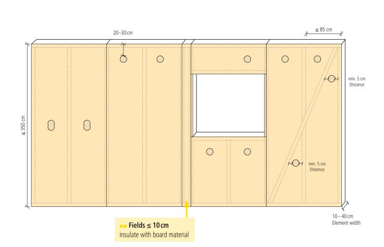
Defined holes 106.5 or 120 mm are only required with cork sealing plugs.
