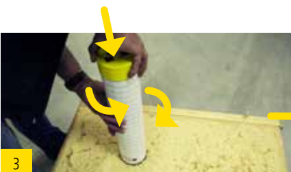
Carefully screw the test pipe into the insulating material using a little pressure
