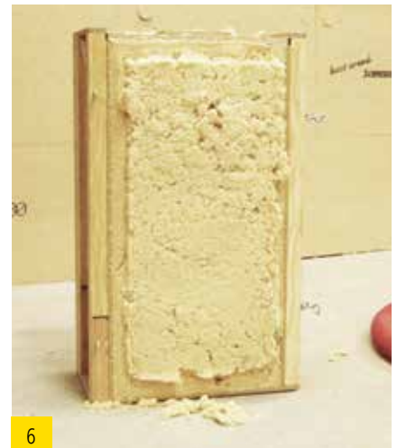
Open test element and assess filling result
