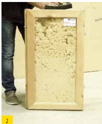
Compacted injection with hose
