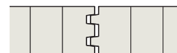
1 cm double tongue and groove Variant 6 Thickness: 45–59 mm Variant 7 Thickness: 60–79 mm Variant 8 Thickness: 80–99 mm
