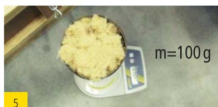
Re-weigh filled test pipe
