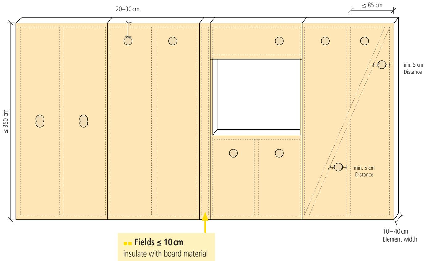
Defined holes 106.5 or 120 mm are only required with cork sealing plugs.
