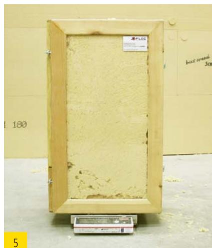
Re-weigh filled test element
