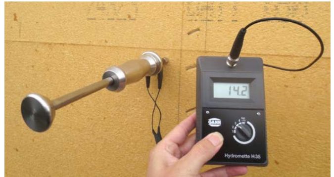
Board moisture content \leq 19.5\% with setting spruce/pine.
