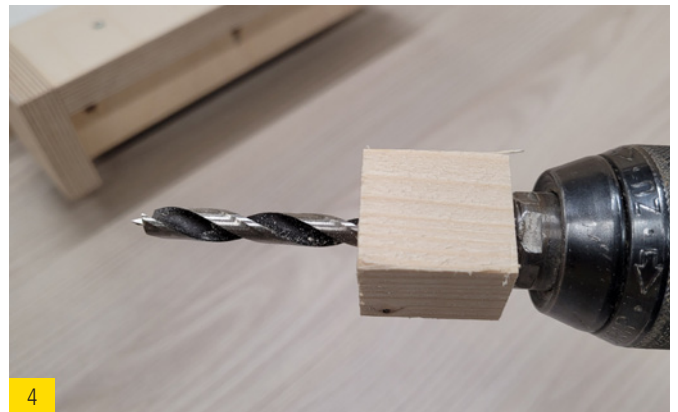
Depth limiter for drilling depth depending on the material thickness of the installation aid. The drill hole must be 22 mm deep.
