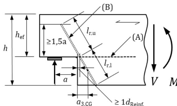
Figure 1-6: Reinforced notched beam support in the ribs of a best wood CLT BOX
