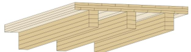
Figure 1-3: Open box with three webs and protruding flange
