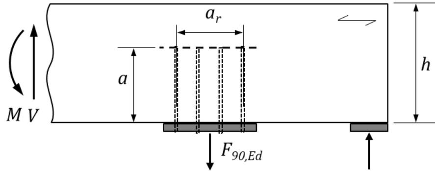
Figure 1-5: Load  $F_{90,Ed}$  perpendicular to grain with possible crack line at the screw tips in the ribs of a best wood CLT BOX
