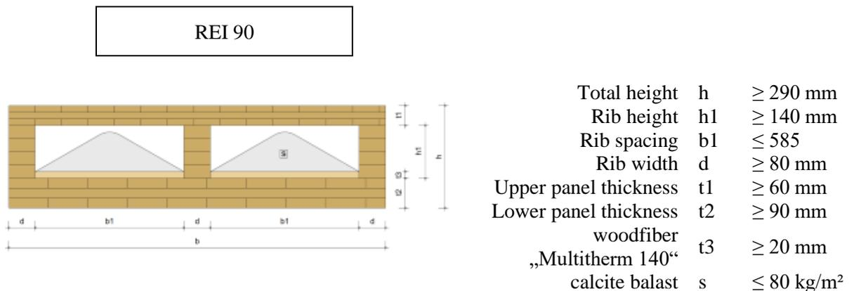
The normal and shear stresses in the glulam ribs and CLT panels must not exceed the relevant stresses in the tested element for REI 90 (width 3756 mm, span 4750 mm, thickness 290 mm) under a uniformly distributed load of 5,5 kN/m<sup>2</sup>.
