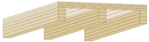
Figure 1-2: Open box with outer webs flush with flange
