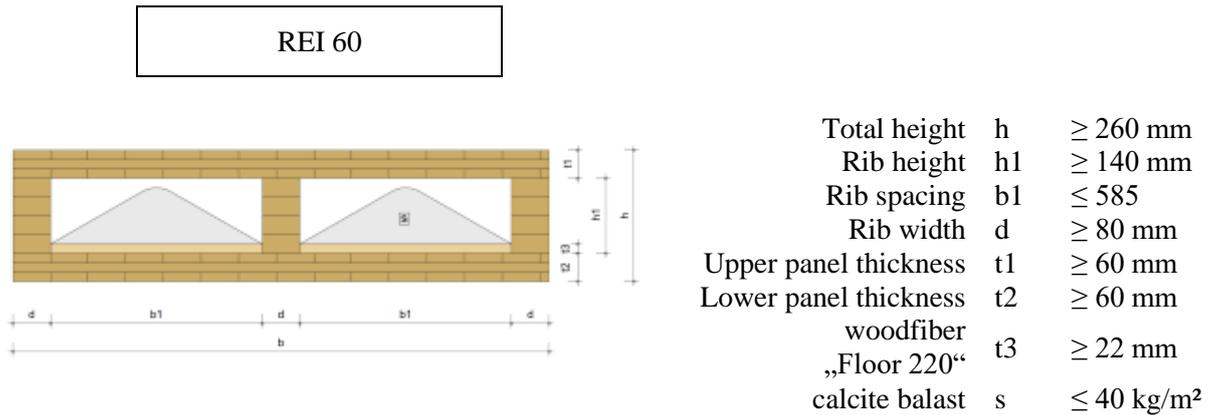
The normal and shear stresses in the glulam ribs and CLT panels must not exceed the relevant stresses in the tested element for REI 60 (width 3756 mm, span 4750 mm, thickness 260 mm) under a uniformly distributed load of 8,0 kN/m<sup>2</sup>.
