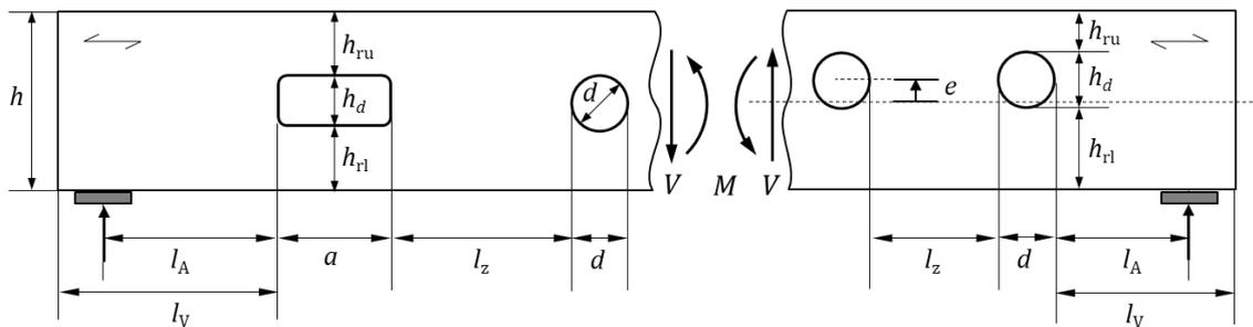
Figure 1-9: Dimensions of holes in the ribs of a best wood CLT BOX
