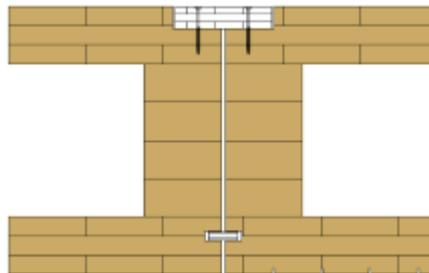
butt joint with screw cross
