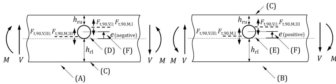
**Figure I-10:** Circular hole in a member with positive (left) or negative (right) bending moment
