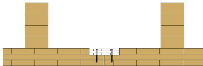
butt joint with screw cross
