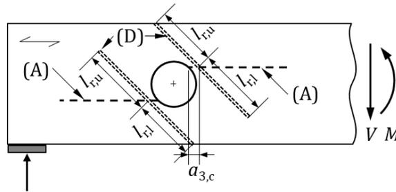
Figure 1-8: Reinforced hole in the ribs of a best wood CLT BOX
