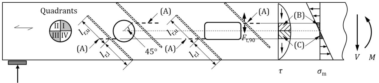
Figure 1-7: Holes in the ribs of a best wood CLT BOX
