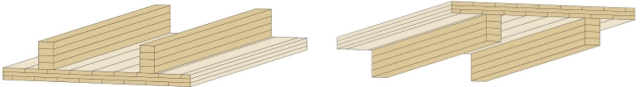
*Figure 1-4: Open box with two webs and protruding flange*
