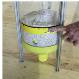
If the chippings are delivered in Big-Packs, pour in the chippings up to the mark = 12.5 kg
