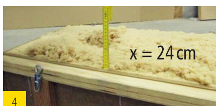
Determine the insulation thickness
