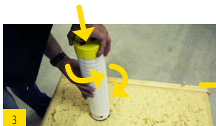
Carefully screw the test pipe into the insulating material using a little pressure
