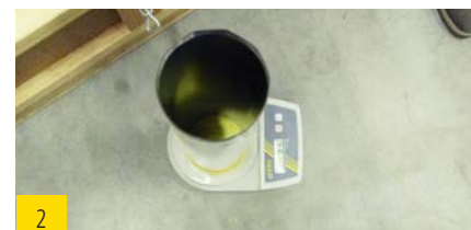
Weigh empty test pipe
