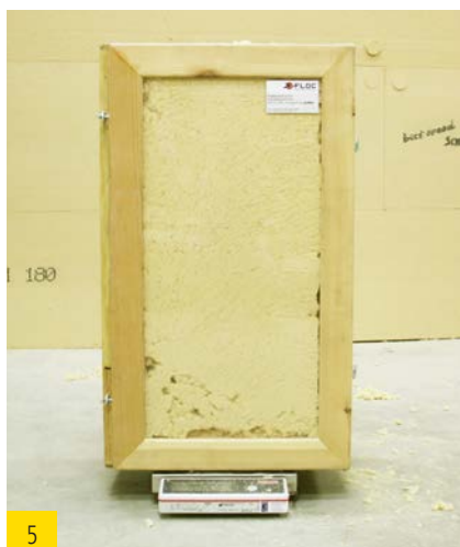
Re-weigh filled test element
