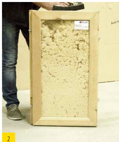
Compacted injection with hose
