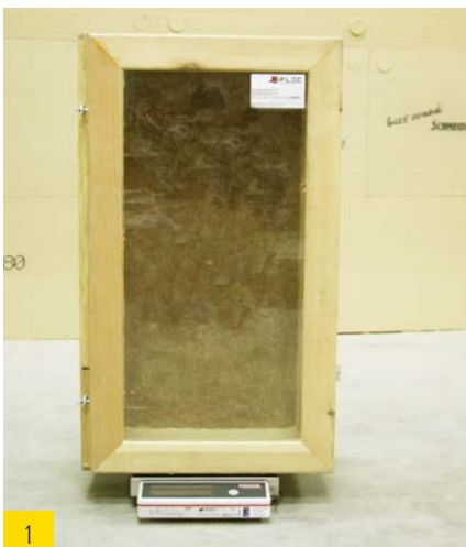
Weigh empty test element
